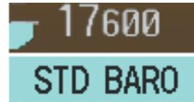
Pressure setting flashes during descent below transition altitude to indicate setting has not been changed from STD BARO.
