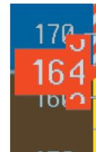
Figure 2-4 Red Pointer Showing Overspeed (Model 172R)
