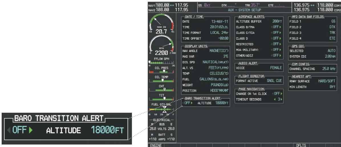
Figure 2-10 Baro Transition Alert (AUX - System Setup Page)
