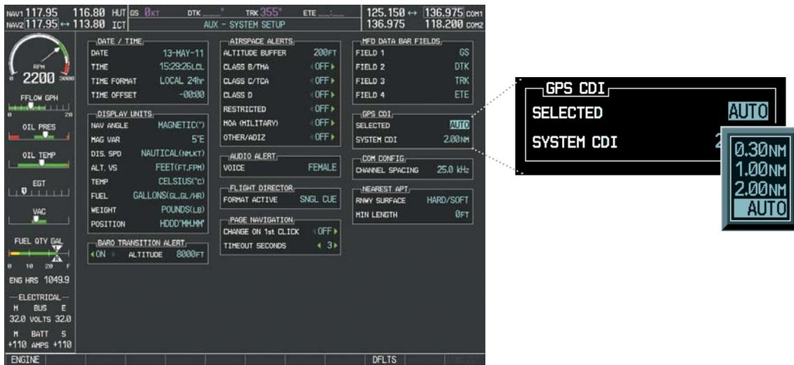
Figure 2-22 GPS CDI Settings (AUX - System Setup Page)
